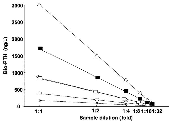
Fig. 4. Linear dilution curves for six sera with different PTH concentrations, as measured by the Bio-PTH assay.
