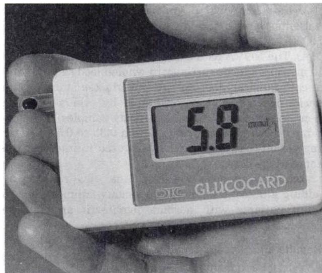
Fig. 1. Glucocard blood glucose test meter with a glucose-electrode control strip
