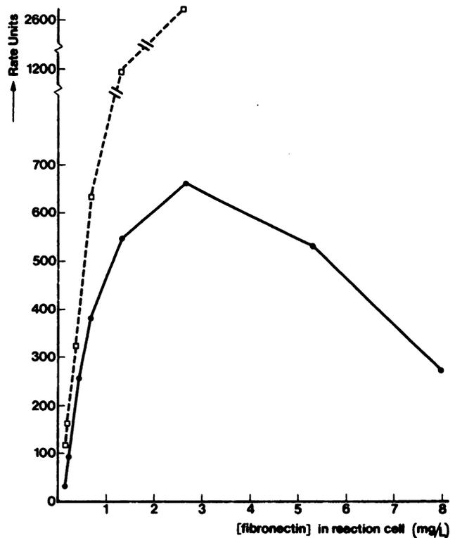
Fig. 2. Relation between the measured rate of change of scatter ("rate units") and the fibronectin concentration in a normal plasma (fibronectin concentration 260 mg/L) diluted two- to 108-fold and assayed with antiserum diluted 21-fold (●) and sevenfold (□)
