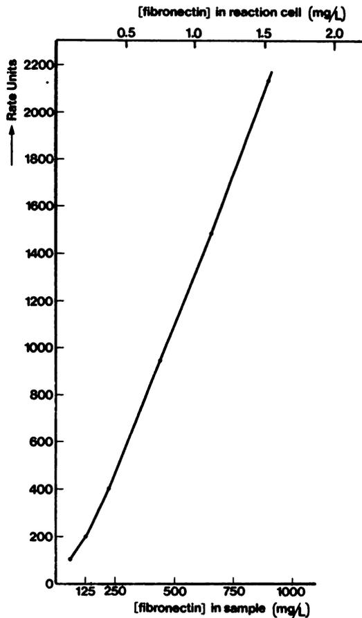
Fig. 1. Standard curve for fibronectin, obtained with anti-human fibronectin antiserum from rabbit, diluted sevenfold with PBS, and fibronectin standards of 125, 250, 500, 750, and 1000 mg/L, diluted 36-fold in PBS
