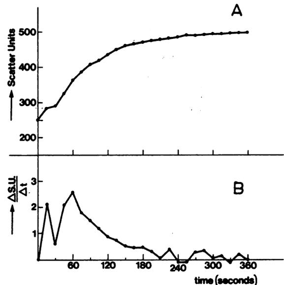
Fig. 3. Course of antigen-antibody complex formation, determined with the Beckman ICS in the "scatter mode," for a normal plasma sample (fibronectin concentration 288 mg/L) reacted with antiserum diluted fivefold
