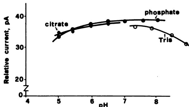
Fig. 1. pH and buffer effect on the new L-lactate sensor. On adding L-lactate to give a final concentration of  $1 \times 10^{-4}$  mol/L the oxygen current decreased; the variation is reported on the y-axis as relative current (percentage of saturation value)
