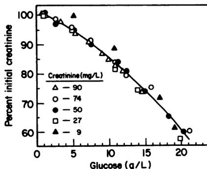
Fig. 1. Creatinine inhibition on the Ektachem by high serum glucose
