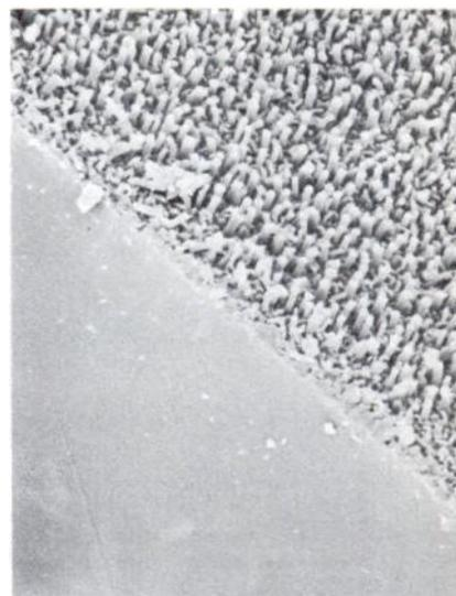
Fig. 1. Electron-scan micrograph of silica filaments on the walls of wide-bore Pyrex glass tubing
