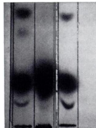
Fig. 9. Thin-layer chromatography of lipids. Silica Gel F<sub>254</sub>, hexane:diethylether:acetic acid (80:20:1.5, by vol)
