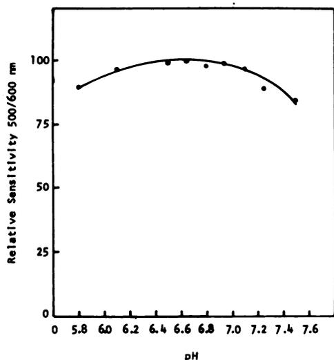
Fig. 6. Effect of pH on final absorbance
