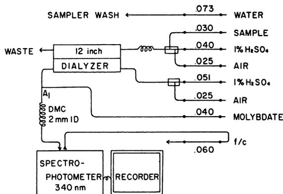
Fig. 1. Manifold diagram for serum phosphorus analyses
