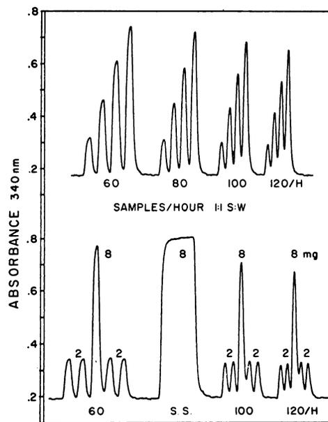
Fig. 2. Beer's law is obeyed at sampling rates of 60 to 120 samples/hour. Sample carryover is negligible, as shown by the sequences of low-high-low peaks. Steady state (s.s.) is readily attainable
