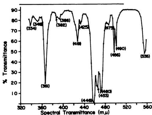
Fig. 1. Spectral transmittance scan with holmium oxide filter in Beckman DU spectrophotometer. Parentheses indicate true wavelength.
