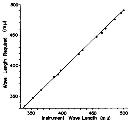
Fig. 2. Graph for correcting instrument (wavelength) setting to true wavelength.
